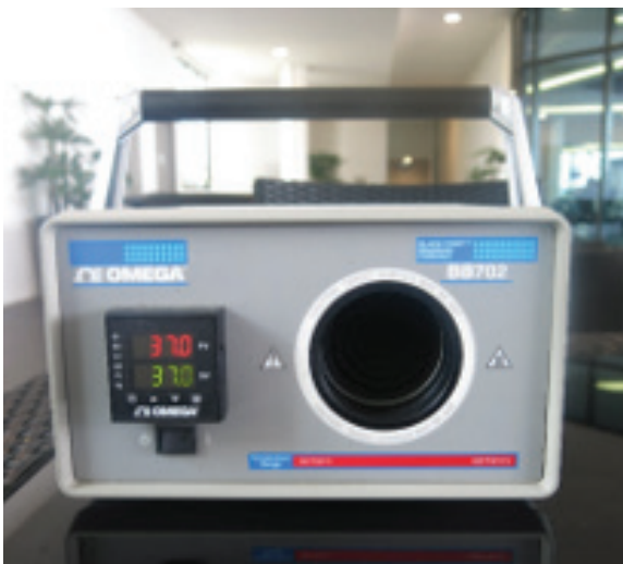
Figure 4. Example of a Blackbody Cavity
