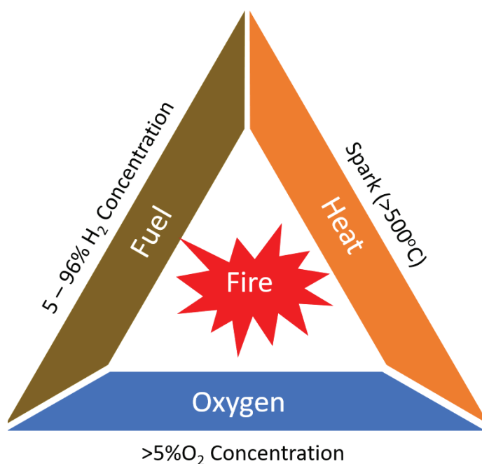
Figure 3. Fire Triangle Required for Combustion
