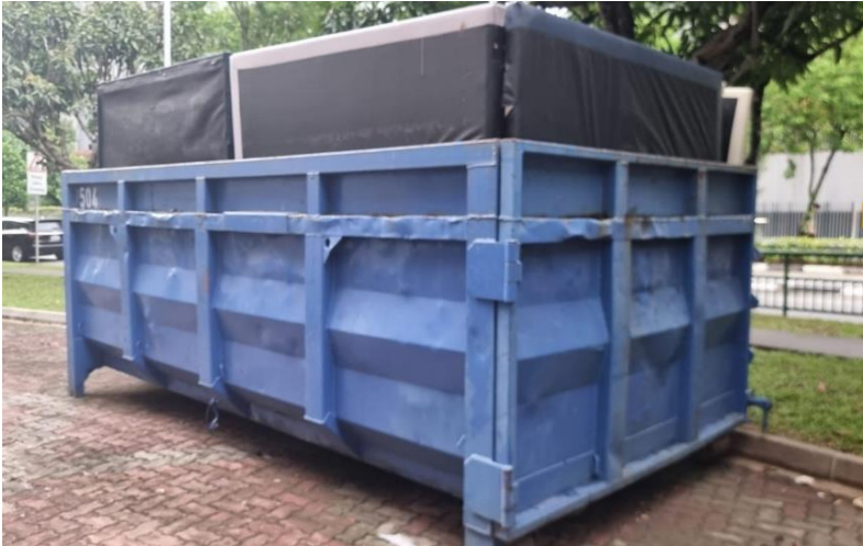
Figure 1 The side wall height of the OTC was extended using boards, which is unsafe.
