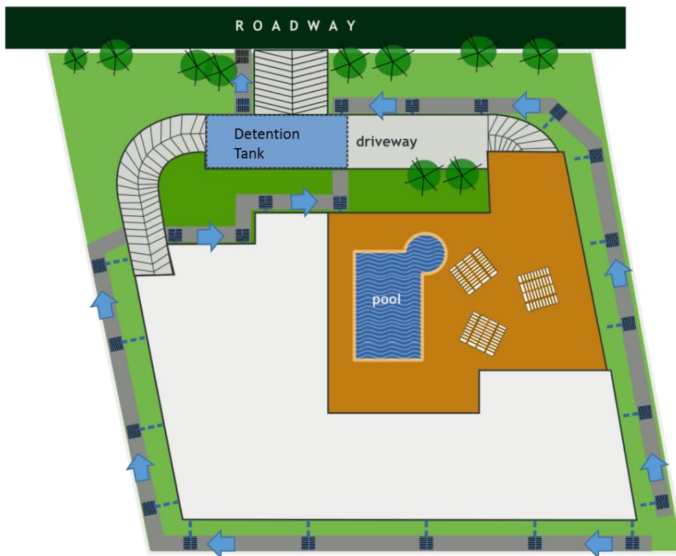
Figure 7.1.2: Location of Detention Tank
