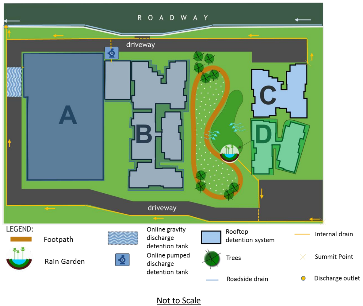
Figure 7.3.2: Locations of Detention Systems
